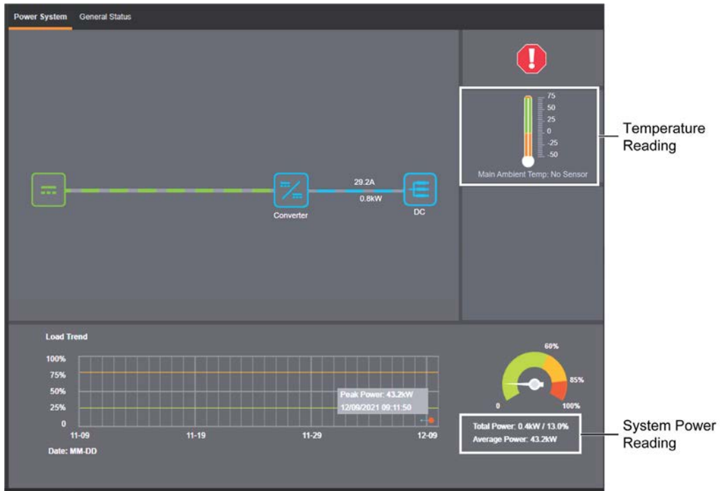
Figure 9-9 Power System Status Tab
